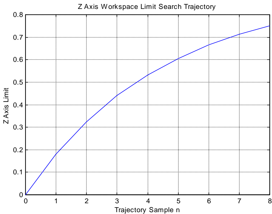
Figure 3.2 Z Axis Upper Limit Search Trajectory
