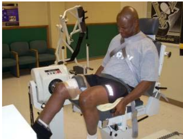
Figure 9. Knee Flex/Ext Strength Testing
