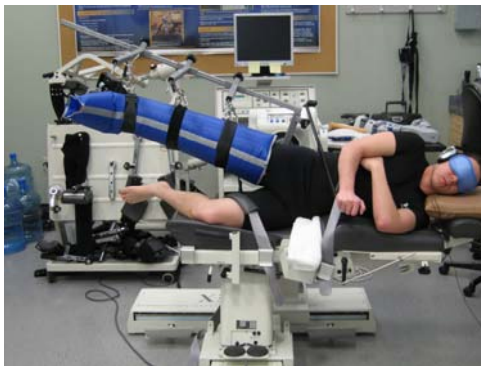
Figure 9. Testing set up for abduction / adduction TTDPM
