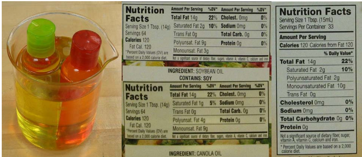
Figure 3-9 Imaging Phantom Constructed with 3 Types of Oil and Their Package Labels
