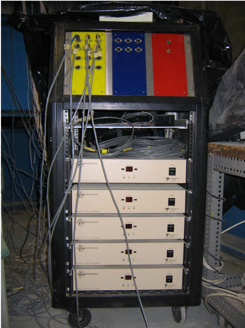
Figure A 10 Data Acquisition System
