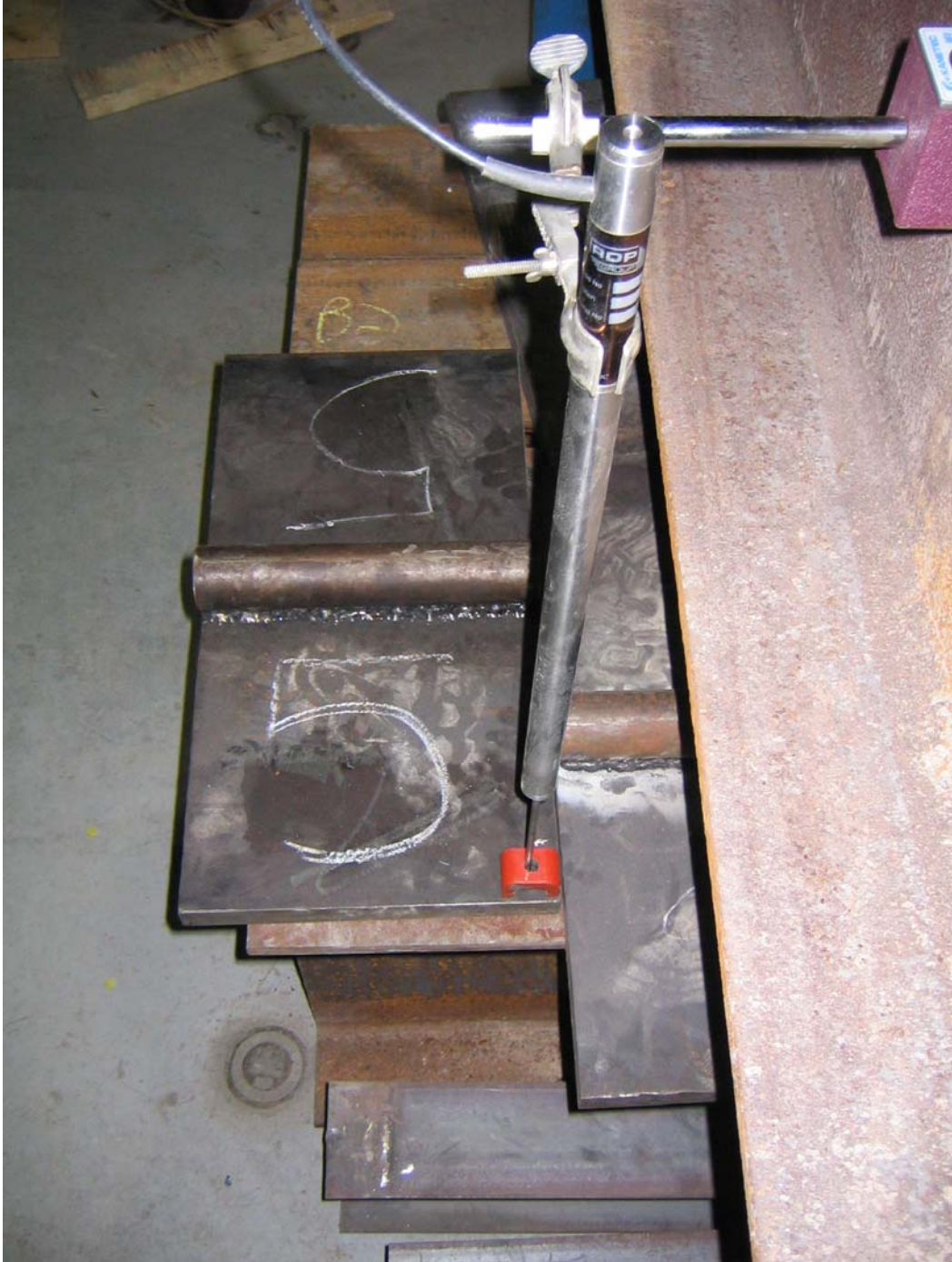
Figure A 9 Representative Layout of DCDT Placement on HS25-44 Steel Test Plate
