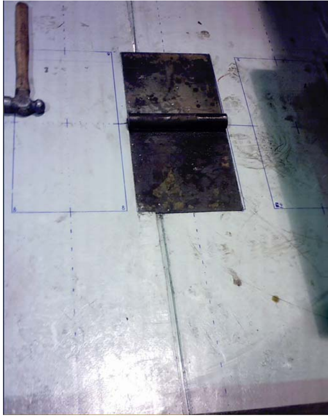
Figure 2.14 Damage Caused By the Embedded Steel Test Pad After Completion of Test 6
