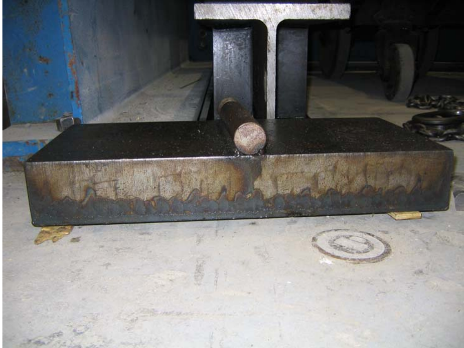
Figure 2.6 Three-inch Thick Steel Test Pad
