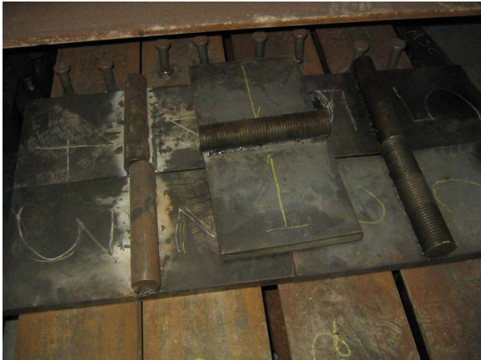
Figure 2.5 The One-inch Thick Steel Test Pads Used For Testing Positions 1 Through 5
