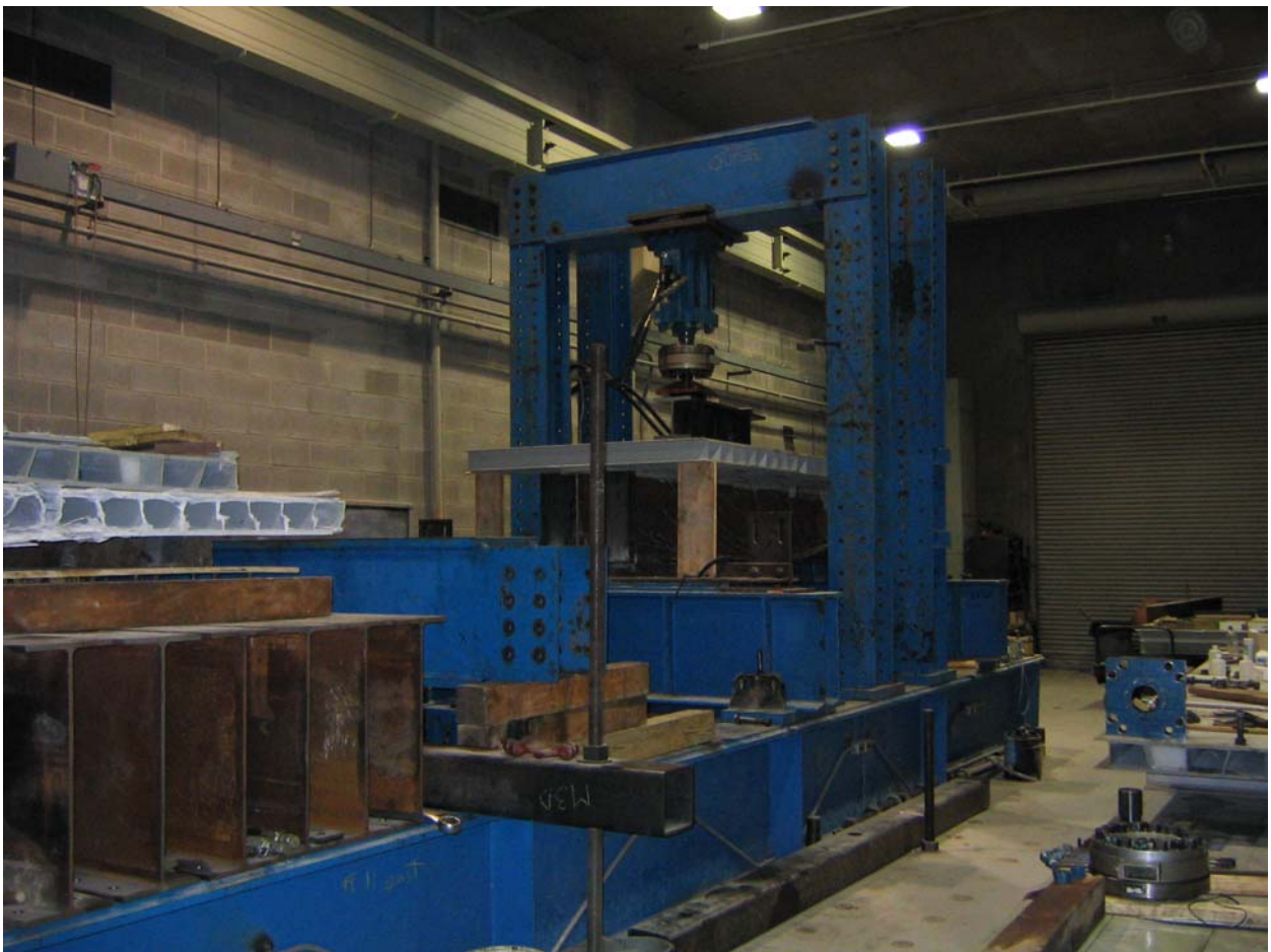
Figure A 5 Overview of Load Frame After the End of Testing
