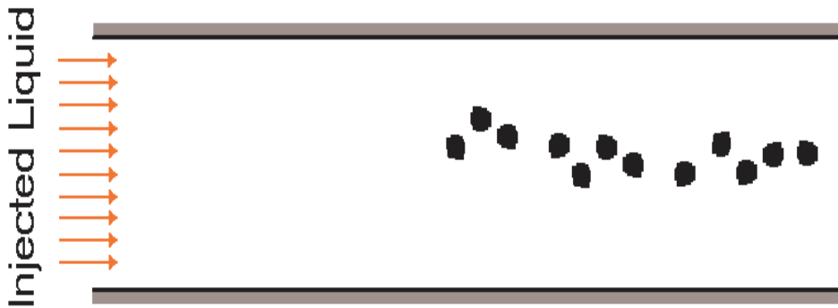
Figure 1.3. Motion of debris along the flow in a polymeric liquid.
