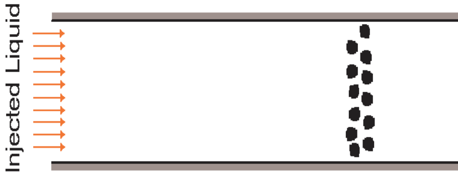
Figure 1.2. Motion of debris across the flow in a Newtonian liquid.
