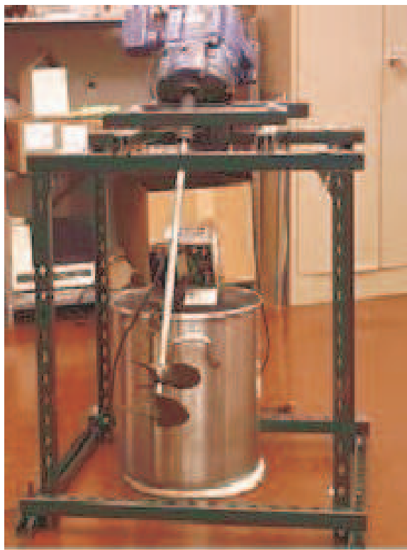
Figure 6.3. A snapshot of the mixer and mixing vessel used to prepare the polymer.
