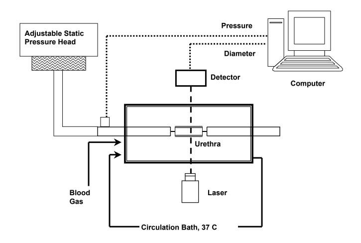
Figure 2.1: A schematic of the modified ex vivo urethral testing system
