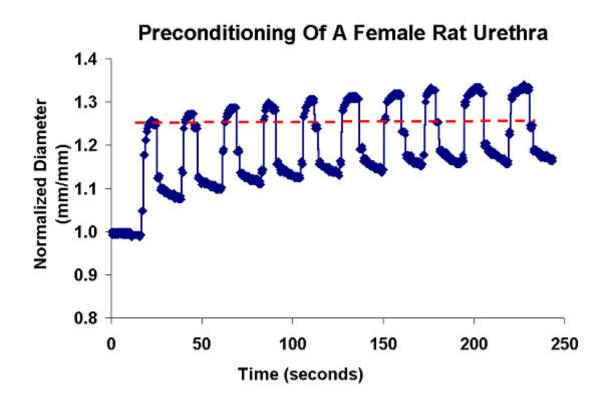
Figure 2.3 : The above picture represents the results of the preconditioning regimen of the middle region for a female rat urethra in the baseline state. The dotted line indicates the diameter of the urethra after the first cycle's pressure step, illustrating the change in peak diameter over from the first cycle to the tenth. Note that by the sixth or seventh cycle the cycles begin to appear repeatable.
