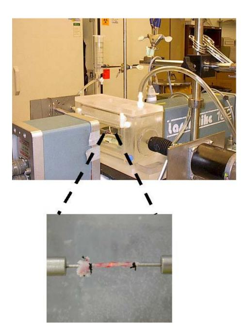
Figure 2.2: A photograph of the entire testing system (top), and a female rat urethra mounted onto the attachment/infusion tees (bottom). The urethras tested had an average length of approximately 20mm.
