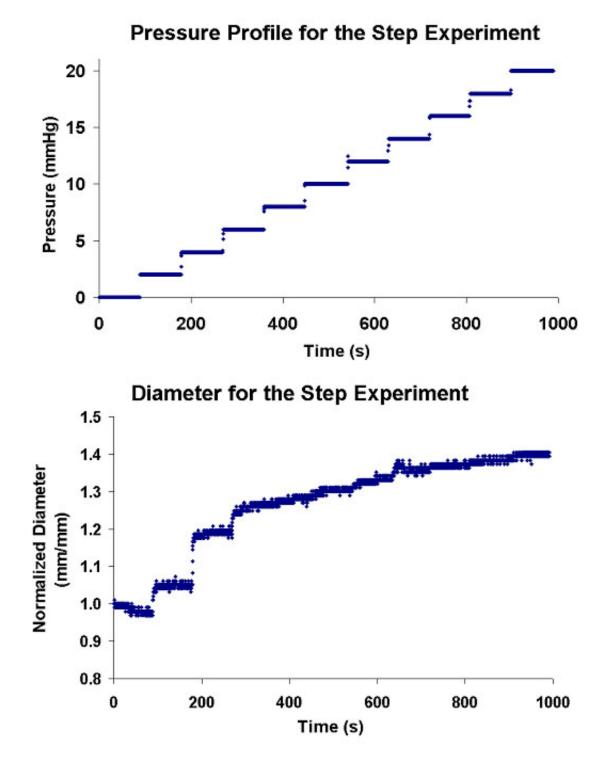
Figure 2.4: *Top*: The pressure profile for a static pressure experiment holding each increment of pressure for 5 minutes. *Bottom*: The resulting outer diameter measurement for the proximal portion of a female rat urethra.
