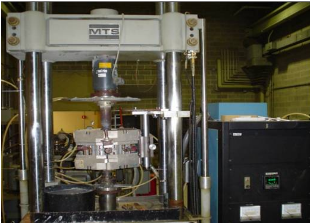
Figure 4.2: MTS hot compression system at BAMPRI labs in the University of Pittsburgh.
