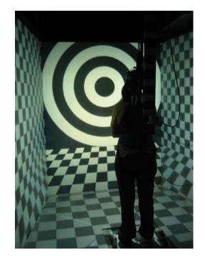
Figure 2 Subject viewing a bullseye-and-checkerboard pattern in the BNAVE virtual environment. Sway responses were recorded via a single force plate beneath the feet, and an electromagnetic tracking device located at the head. Subject is secured to the support structure by a safety harness.
