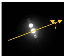
Figure 44. Nano-diffraction pattern including the rotation axis over which regions in the area are misoriented
