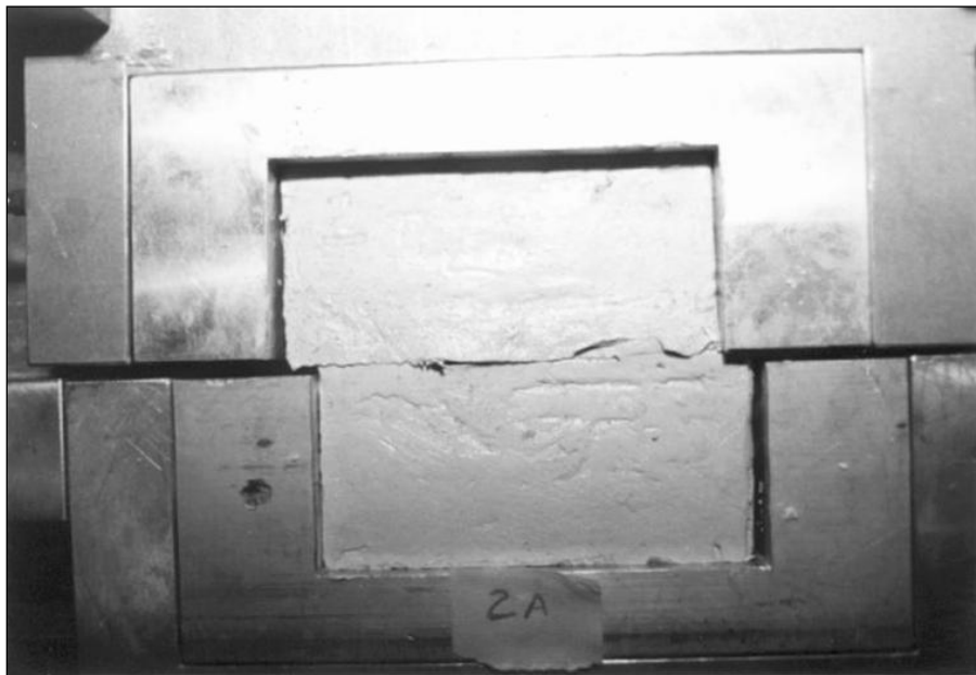
b) Shear displacement = 0.65 cm, near conclusion of test.
