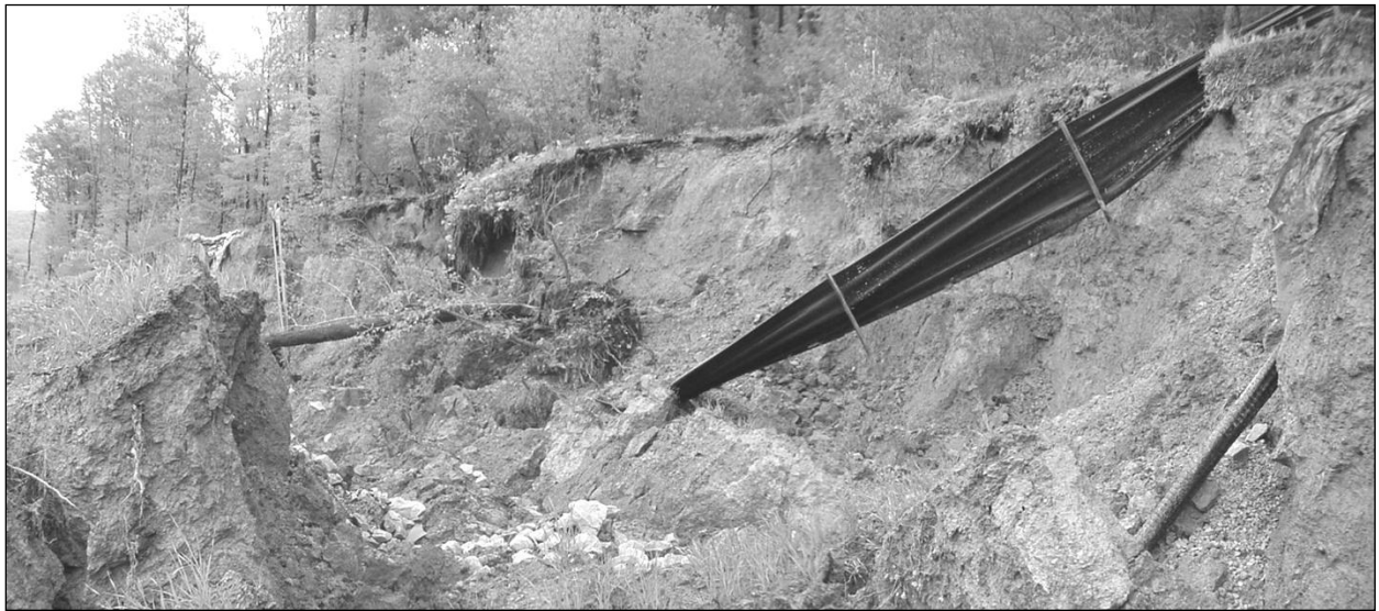
(b) View of 7.6 meter tall main scarp.
