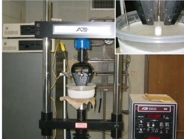
Figure 26. Photograph of the pseudo-Bridgman solidification apparatus with inset detail of the sample being immersed into the freezing bath.
