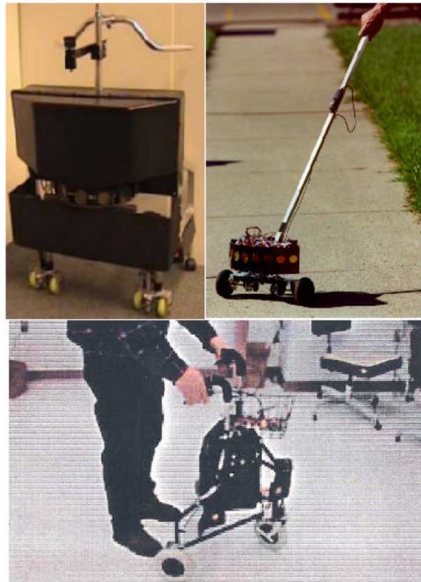
Figure 12 Clockwise from the top left: The PAMM smart-walker developed at MIT; The GuideCane invented at the University of Michigan; The assistive robotic walker designed at the University of Virginia Medical Center.
