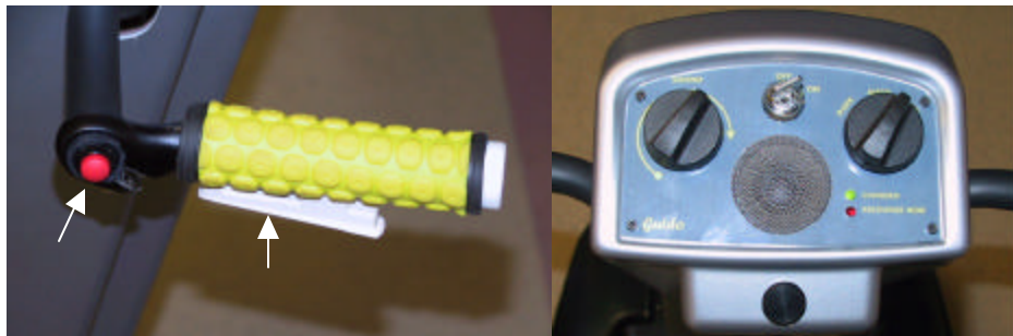
Figure 4 The picture on the left shows the walker handgrip. The arrows are pointing to the red turn buttons and the white brake lever. The photo on the right shows the control console of the device.
