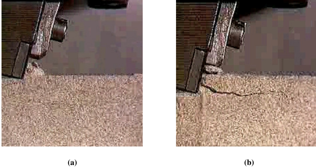
Figure 2.3 The Rock Scratching Test: (a) a ductile failure mode and (b) a brittle failure mode
