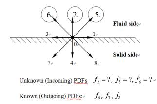
Figure 2.4: PDFs of a flat boundary site at the lower wall boundary after the streaming
