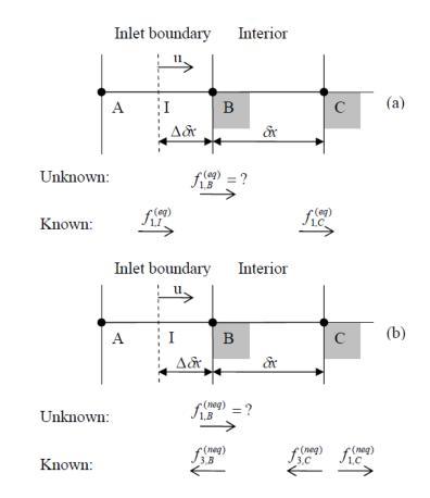
Figure 2.6: Configuration of PDFs used to construct the inlet boundary condition: (a) Configuration of equilibrium PDFs at the inlet, (b) Configuration of non-equilibrium PDFs at the inlet (the gray color denotes a fluid node)
