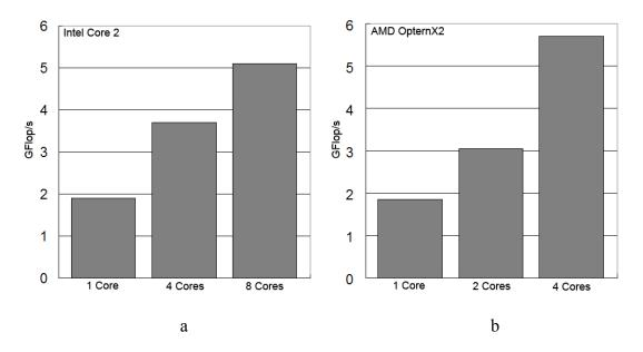
Figure 5.1: Comparison of runtime performance for a different number of cores on a 64X64X64 LBE problem<sup>38</sup> for the (a) Intel Core 2 and (b) AMD OpternX2
