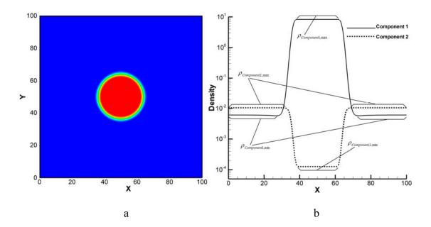
Figure 4.1: (a) Density contour for a circular droplet, (b) Comparison of the densities of the two components along the center line (y = 50,  $0 \le x \le 100$ )
