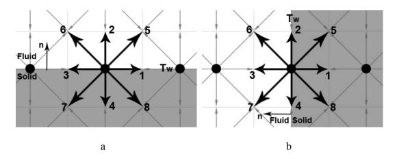
Figure 2.7: Sketch of thermal boundary condition for D2Q9
