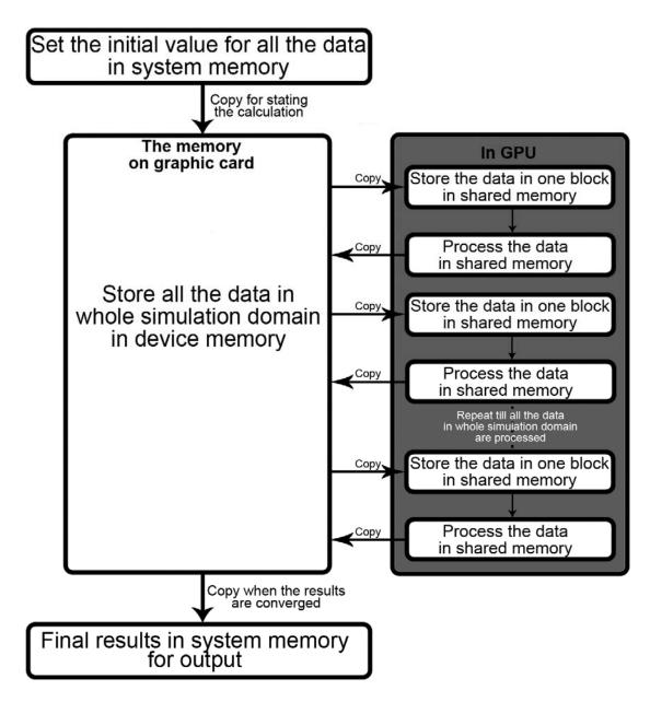
Figure 5.8: General programming strategy for numerical simulation based on CUDA
