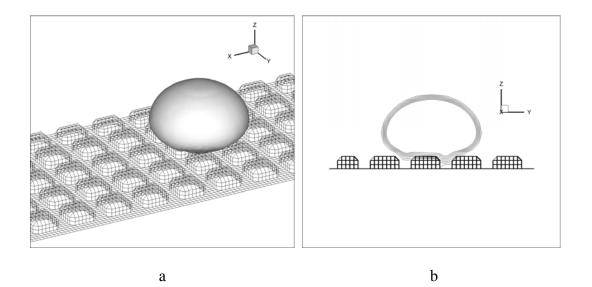
Figure 5.26: (a) liquid droplet on hydrophobic surface, (b) a cross section of droplet
