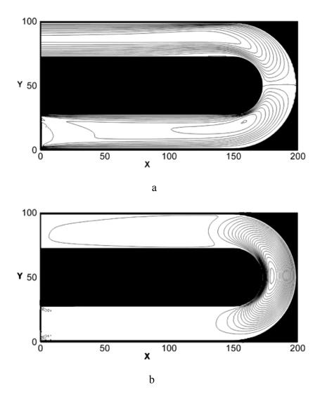
Figure 3.2: Flow in a curved pipe (a) x-velocity contour and (b) y-velocity contour
