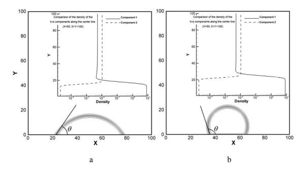
Figure 4.8: Position of the interface of the two components on a hydrophilic and hydrophobic surface, and comparison of the density of the two components along the center line
