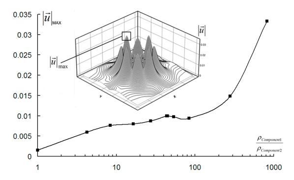
Figure 4.6: The maximum magnitude of the spurious currents varying with the density
