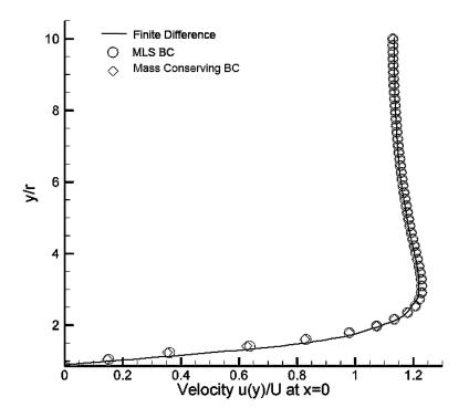
Figure 3.6: Comparison of the velocity profiles at x=0 for the MLS BC, mass conserving
