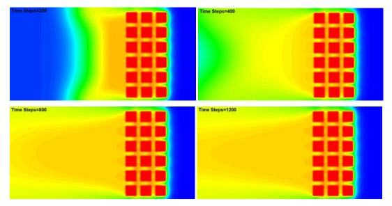
Figure 5.23: Temperature contour at the slice of y=20 for time steps 200, 400, 800 and
