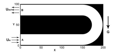
Figure 3.1: Schematic computational area for flow in a curved pipe
