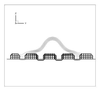
Figure 5.29: A cross section of droplet on hydrophilic surface
