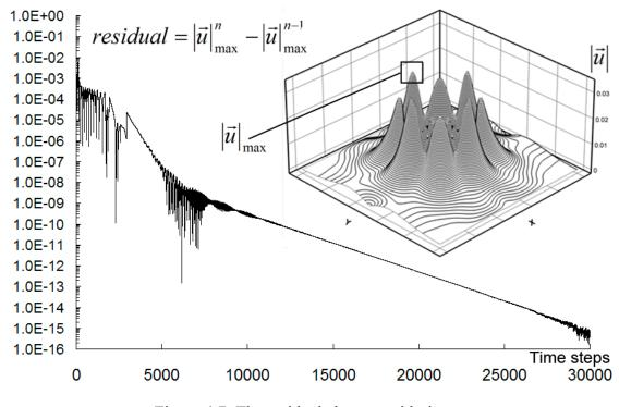
Figure 4.7: The residual changes with time steps
