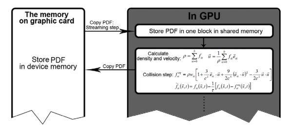
Figure 5.12: Demonstration of the streaming step and collision step based on the CUDA LBE model
