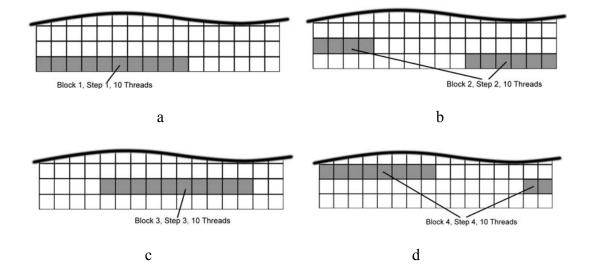
Figure 5.10: Demonstration of block division for CUDA
