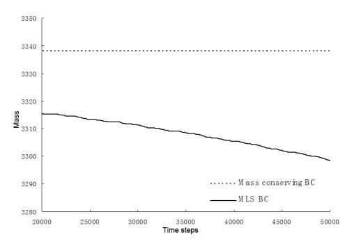
Figure 3.3: System mass change with time using the mass conserving BC and MLS BC
