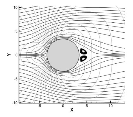
Figure 3.5: Steady flow around a cylinder at Re=10, with streamlines and pressure
