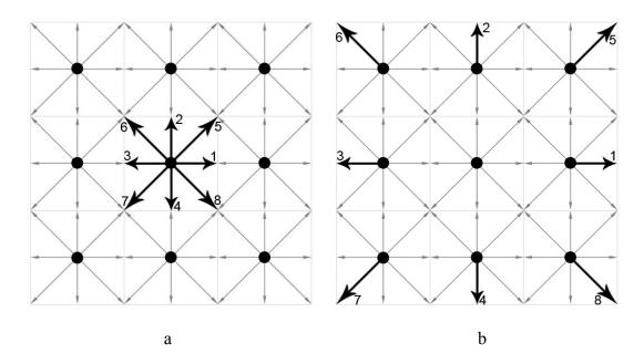
Figure 5.11: Streaming step: (a) time step 0; (b) time step 1
