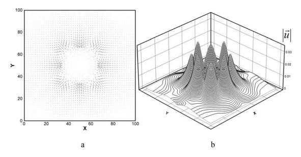
Figure 4.5: (a) Vector of spurious current around the droplet, (b) magnitude of the spurious current
