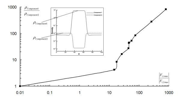
Figure 4.4: Density ratio  $\frac{\rho_{Component1}}{\rho_{Component2}}$  variation with the ratio of the maximum force
