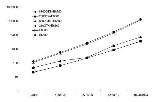
Figure 5.17: Calculation time comparison between GPUs and CPUs
