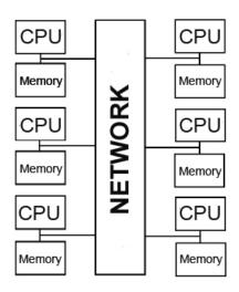
Figure 5.3: Modern supercomputer architecture
