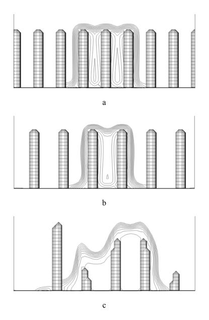
Figure 5.34: Cross section of droplet for different distribution of pillars, (a) distance between pillars is 4 grids, (b) distance between pillars is 8 grids, (c) pillars have different lengths
