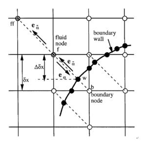
Figure 2.3: Layout of the lattice and curved wall boundary
