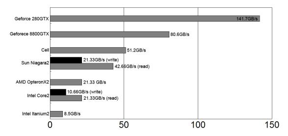
Figure 5.7: Comparison of memory bandwidth for different system
