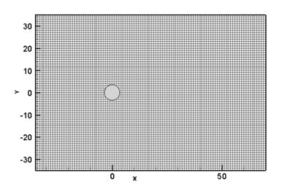
Figure 3.4: Schematic of the computational area for steady flow over a circular cylinder. The cylinder has a diameter of 7 lattice units. The cylinder center-to-center distance (H) is 70
