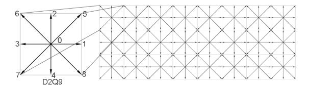
Figure 1.1: The 2D grids for LBM
