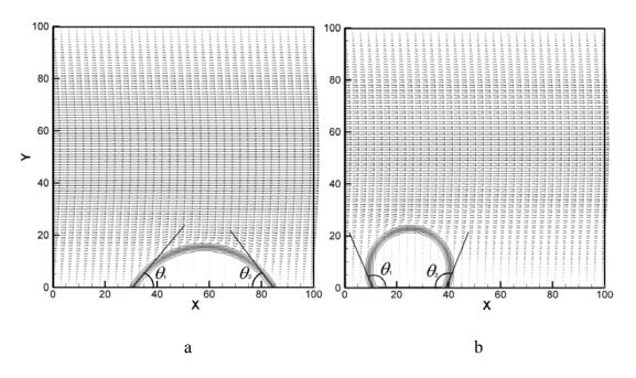
Figure 4.9: Position of interface of the two components and velocity vector,
