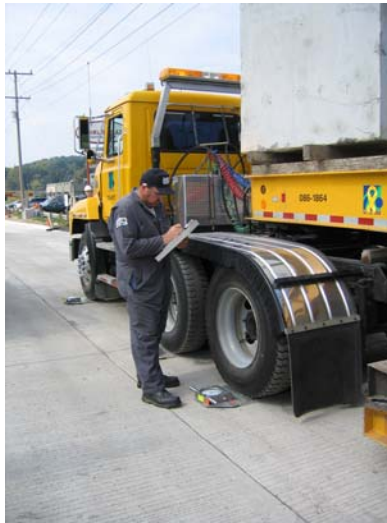
Figure 5.2. Verification of axle loads.
