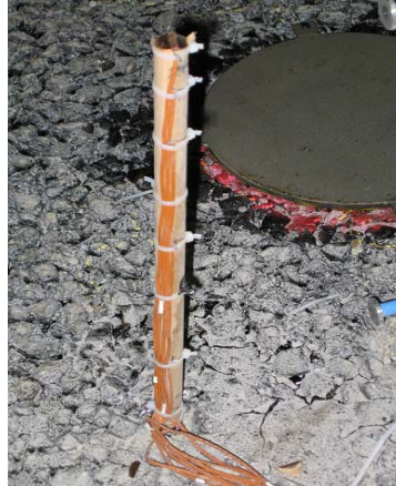
Figure 3.5. Thermocouples used to measure temperature throughout the pavement (Wells et al. 2005).
