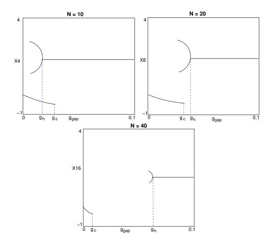
Figure 3.4.3: Sketches of bifurcation diagrams for various N values.  $g_c$  is the value of  $g_{gap}$  where the two-cluster state becomes unstable and  $g_h$  is where the Hopf bifurcation is observed. For N=10,  $g_c=0.02759$ ,  $g_h=0.001823$ ; N=20,  $g_c=0.003491$ ,  $g_h=0.007463$ ; N=40,  $g_c=0.003771$ ,  $g_h=0.03045$ .
