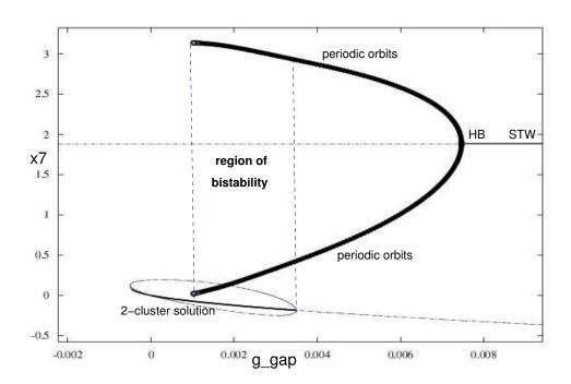
Figure 3.4.2: Bifurcation diagram as  $g_{gap}$  varies for a system with 20 oscillators. Two-cluster state becomes unstable at  $g_{gap} = 0.003491$ . Branch of solutions bifurcating from two-cluster state are drawn. Traveling waves become unstable through a Hopf bifurcation at  $g_{gap} = 0.007463$ . The periodic orbits are stable and they terminate at a homoclinic point. There is a region where both the two-cluster state and periodic orbits are stable.
