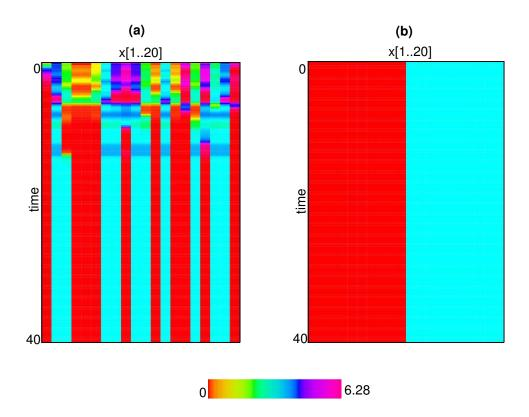
Figure 3.4.1: Two-cluster solution in a network with 20 oscillators where  $x_j = \theta_j - \theta_1$ .
