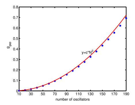
Figure 3.3.1: Relation between  $g_{gap}$  and N is shown by the blue \*'s. The red line is the curve that fits the data with  $y = cN^2$  and c = 0.00002.  $g_{syn}$  is fixed at 0.1 throughout the computation.
