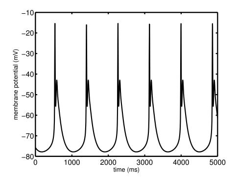
Figure 2.2.1: Uncoupled bursting cells oscillate with a frequency ranging from 0.8 Hz to 1.5 Hz depending on the value of leak potential. Here  $E_{leak} = -82$  mV and the period of the oscillations is about 860 ms.
