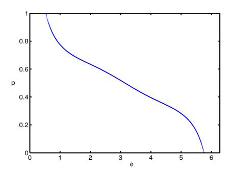
Figure 3.2.1: Possible values for p are graphed as the phase difference,  $\phi$  varies from 0 to  $2\pi$
