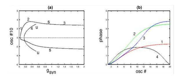
Figure 2.6.4: Behavior of 20 phase oscillators in a *line* as the synaptic coupling increases.(a) The relative phase of oscillator 10;  $g_{gap} = 1$  and the interaction functions are same as in the ring model, (b) Spatial profiles with various solutions from (a). u refers to the solution being unstable and s means the solution is stable.
