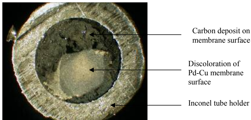
Figure 9. Photograph of the Pd 80wt% Cu membrane after exposure to CO. Conditions: 623 – 1173K, 0.62 and 1.55 MPa. Testing concluded after re-exposure of membrane to 50%H 2 -CO feed at 908K and 0.62 MPa.
