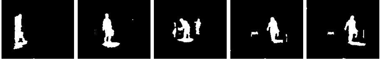
Figure 24: The detected CDM's from the sample frames of Hallway sequence, with the parameter values listed in Table 1. The white (“1-pixel”) regions denote “there are significant changes between the test image (containing moving objects) and the reference image (containing merely background scene)”. It is seen that the significant changes caused by the moving subjects and the suitcase being placed in the hallway were well identified.
