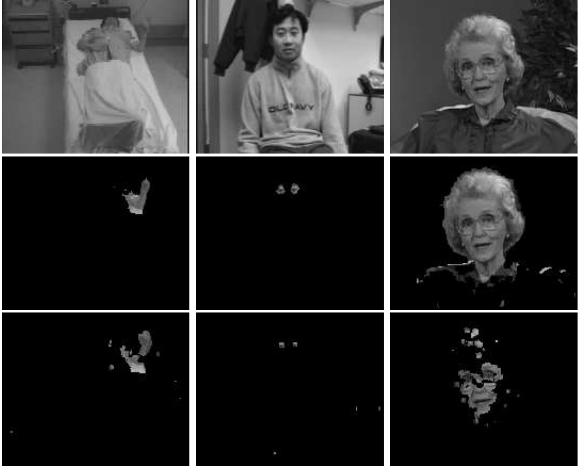
Figure 38: Comparison with significance test method. The top panels show the test frames of patient monitoring video (left), home video (middle), and Grandma sequence (right). The middle panels show the moving objects in the corresponding test sequences, detected by the covariance test method. The bottom panels show the results detected by the significance test method. One may observe from the results that the detection errors, including both the missed detection and the false alarms, were reduced by the covariance test method in contrast to the significance test method.
