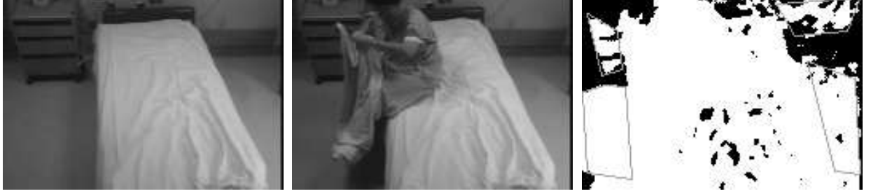
Figure 30: Experimental result on patient monitoring video WITHOUT illumination invariance function. The left panel shows a snapshot of the monitoring unit before the patient’s occupancy. The middle panel shows a sample video frame at the presence of patient. The right panel shows the detected CDM by the proposed method without concerning illumination variation. It is seen that the CDM was affected by the illumination change, for instance, the marked polygonal regions in the background area.
