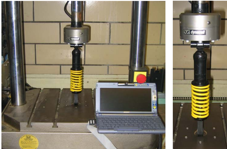
Figure 55 - Instron testing of suspension element for system identification
