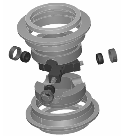
Solid Model of finished SMART CASTER
