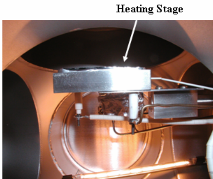
Figure 23 UHV heating stage, (Boraelectric heater used), incorporated in the laser detonation AO source
