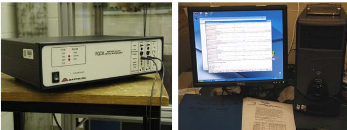
Figure A I- 3 Hardware of Research QCM (Maxtek Inc) system [105]
