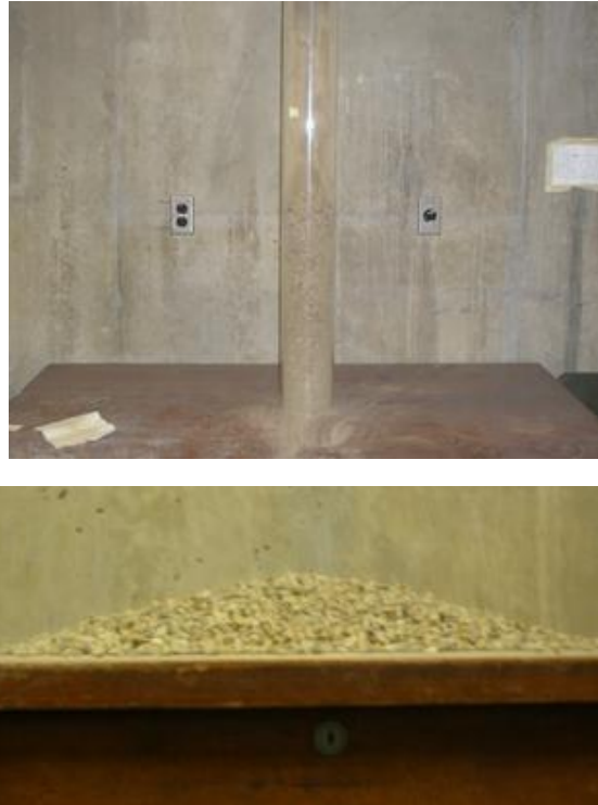
Figure 21. Cylinder experiment (12.5cm inner diameter) with gravel (92.87N) on wood table
