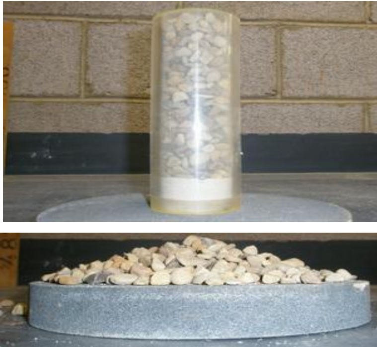
Figure 26. Cylinder experiments using layered system on rough base (2.5cm height sand at bottom), slow velocity
