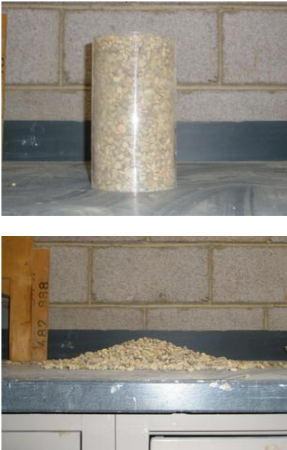
Figure 19. Cylinder experiment (12.0cm inner diameter) with gravel (34.21N), slow velocity
