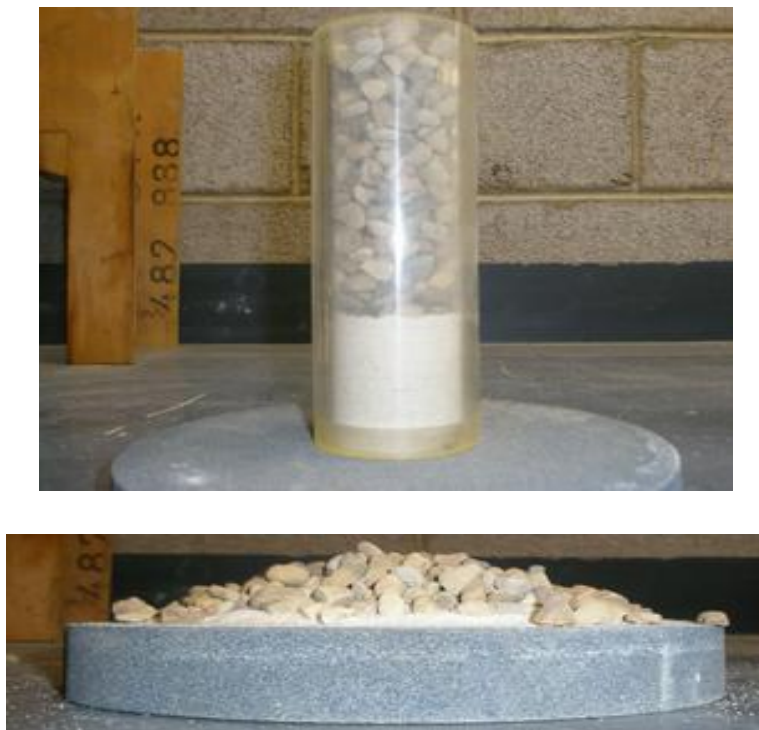
Figure 27. Cylinder experiments using layered system on rough base (5.0cm height sand at bottom), slow velocity
