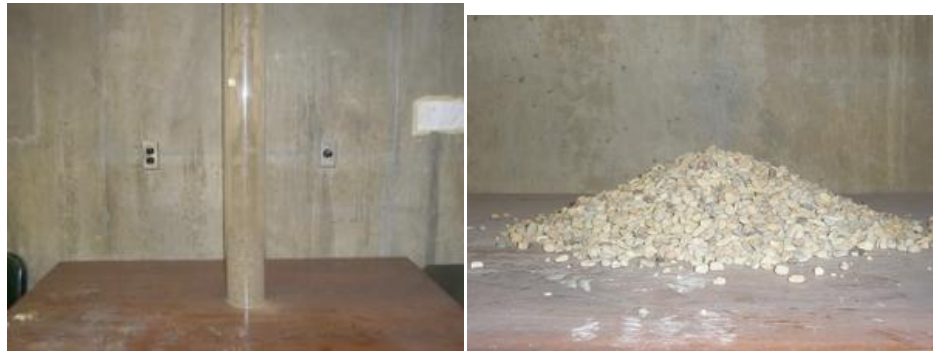
Figure 20. Cylinder experiment (12.5cm inner diameter) with gravel (45.73N) on wood table
