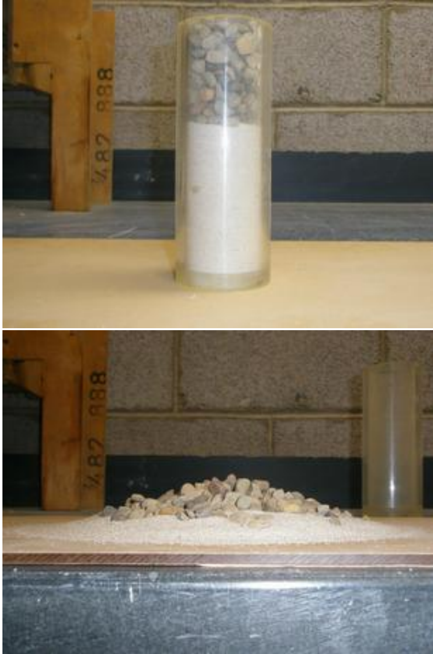
Figure 25. Cylinder experiments using layered system on smooth base (10.0cm height sand at bottom), slow velocity
