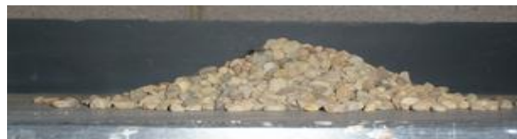
Figure 17. Cylinder experiment (12.0cm inner diameter) with gravel (12.37N), slow velocity
