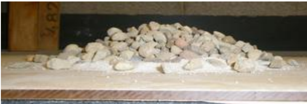
Figure 24. Cylinder experiments using layered system on smooth base (5.0cm height sand at bottom), slow velocity
