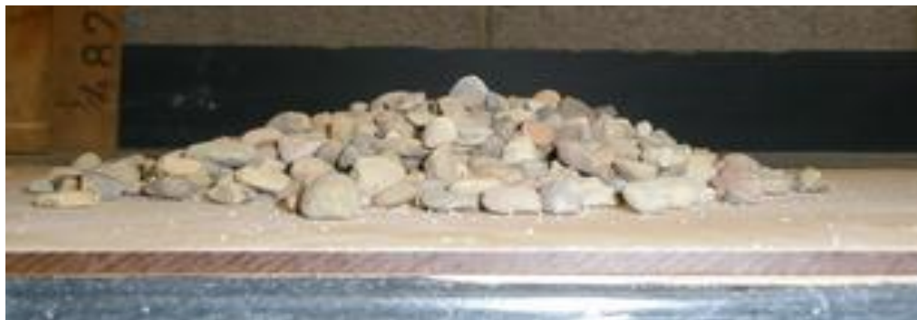
Figure 23. Cylinder experiments using layered system on smooth base (2.5cm height sand at bottom), slow velocity
