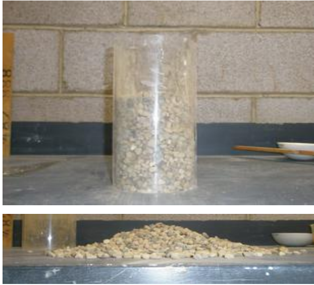
Figure 18. Cylinder experiment (12.0cm inner diameter) with gravel (21.88N), slow velocity
