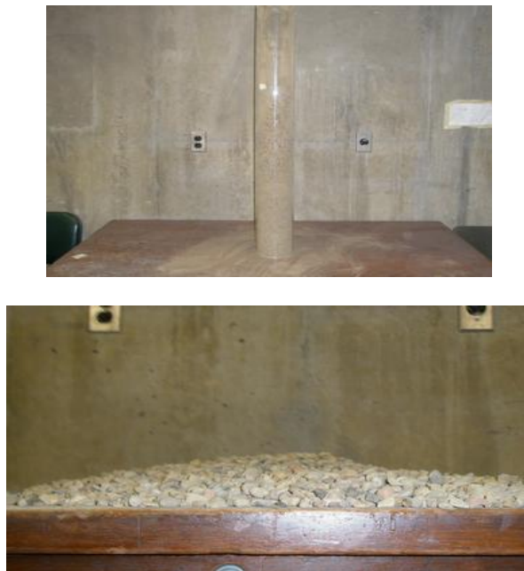
Figure 22. Cylinder experiment (12.5cm inner diameter) with gravel (142.34N) on wood table
