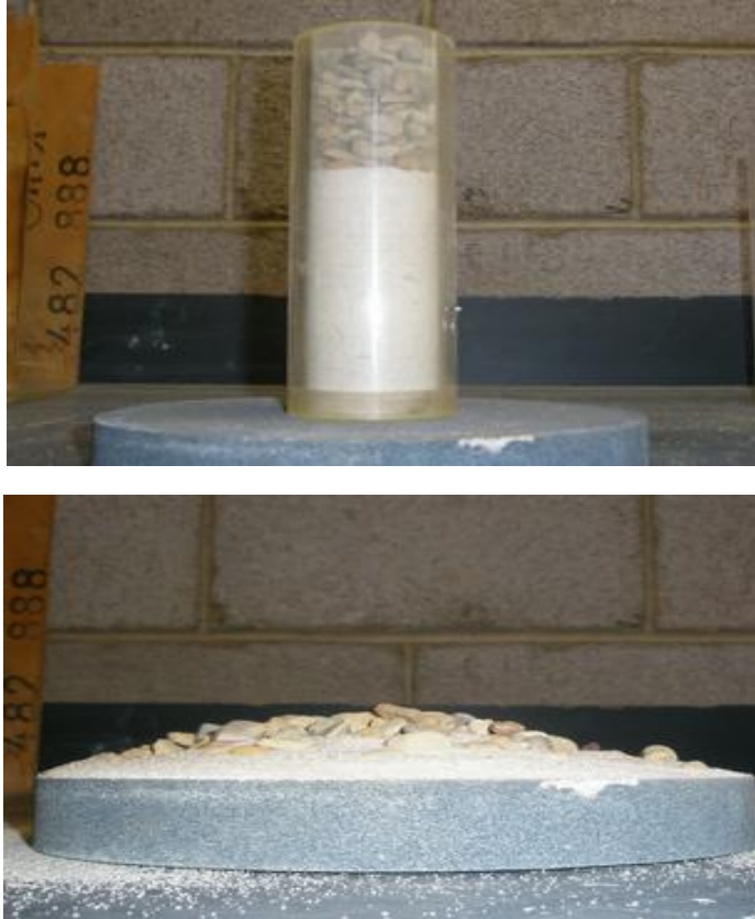
Figure 28. Cylinder experiments using layered system on rough base (10.0cm height sand at bottom), slow velocity
