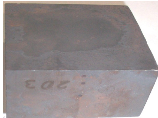
Figure 64 Image of the corrosion on the sample after experiment.
