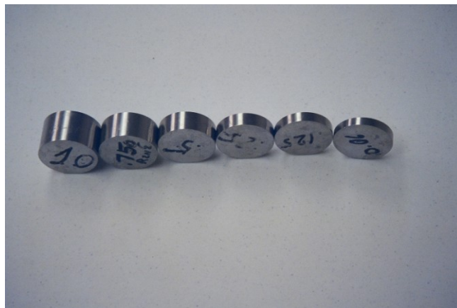
Figure 26 Standard gages to calibrate the sensor for the bottom surface of the tested sample.
