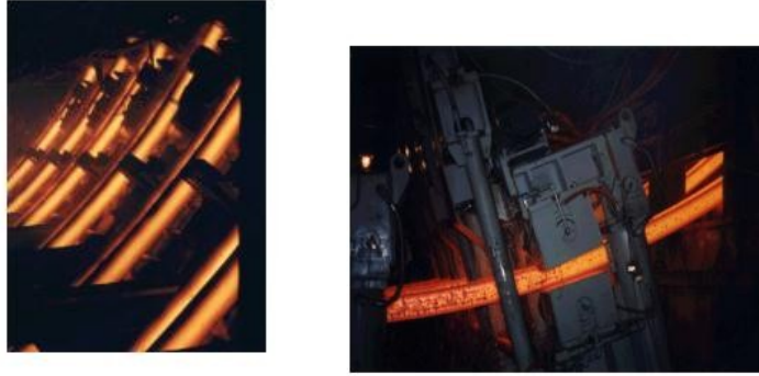
Figure 5 Strand unbending by straightener withdrawal units during secondary cooling zone of continuous casting process of steel [59]
