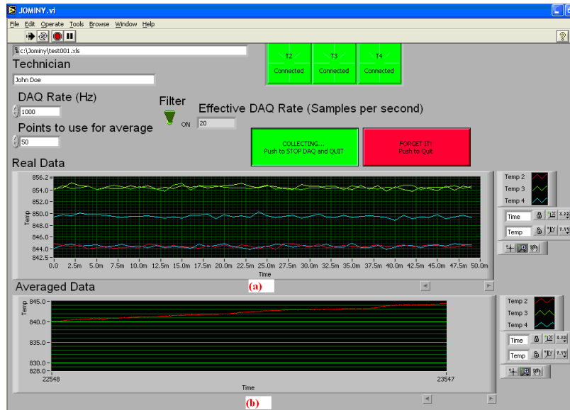
Figure 50 Interface of the Lab view program recoding the data captured by the thermocouple during heating and cooling of the sample; (a) the real time graph (b) time averaging graph; real time graph shows the difference between the thermocouples when they are placed in the furnace without attaching to the sample before the experiment on sample 503B (grade 1319*)
