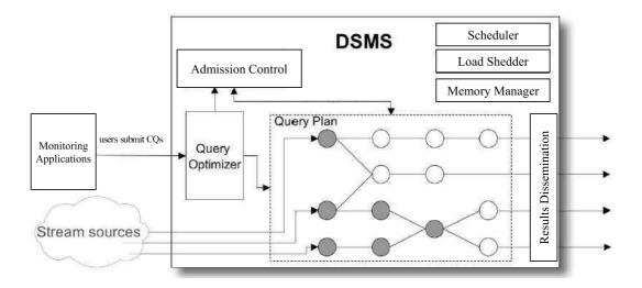
Figure 1: DSMS Architecture.
