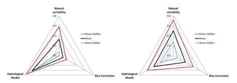
Figure 6: Relative contributions to the uncertainty of 7-day low flow (left) and high flow (right) change in magnitude for the Au Saumon river.
