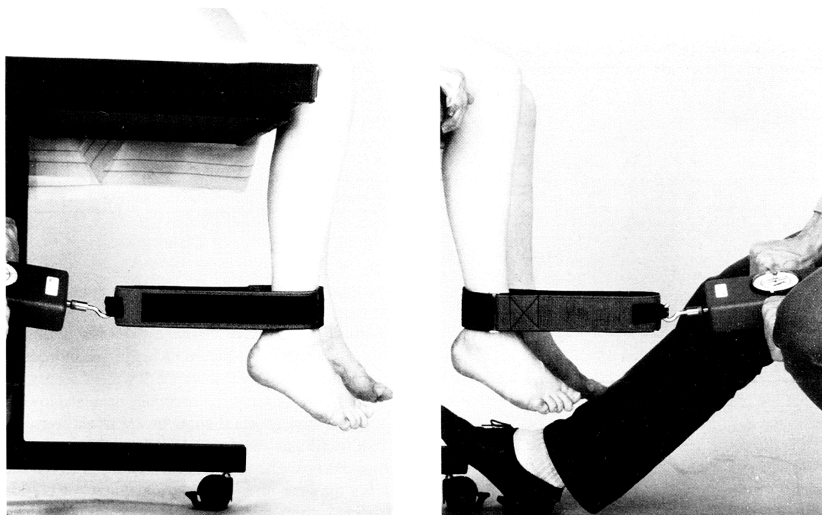
Fig. 1. Measurement of isometric flexion and extension strength of the knee joint with a pull gauge.
