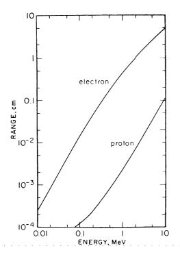
FIGURE 2. Range of electrons and protons in water as a function of energy (ICRU, 1970).
