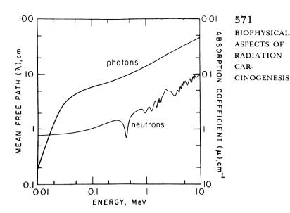
FIGURE 1. Mean free path,  $\lambda(E)$ , and absorption coefficient,  $\mu(E)$ , as a function of energy for photons and neutrons in water.
