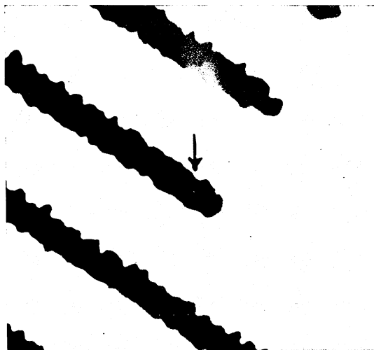
Fig. 2: Production of a fluorescing spot in the object plane by Laser-uv-micro-irradiation. The objective is a Zeiss Ultrafluar 100/1.25 Glyc, and the specimen a Zeiss quartz object micrometer, on which the fluorescing spot is produced. The distance between two lines matches 10\ \mu\text{m} .
