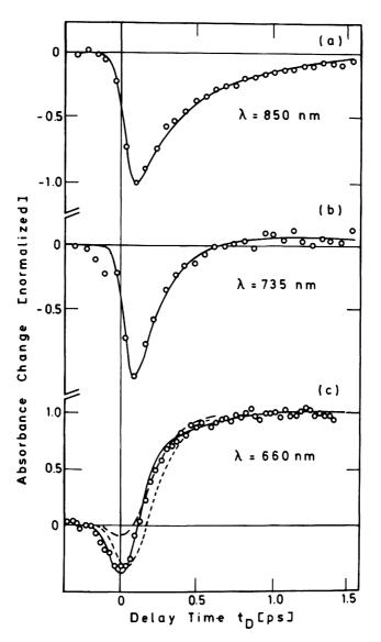
Figure 1. Time-dependent changes of absorption (negative values correspond to gain) induced by exciting femtosecond pulses at  $\lambda = 850$  nm (a),  $\lambda = 735$  nm (b),  $\lambda = 660$  nm (c). The solid curves are calculated using the decay kinetics discussed in the text. The broken curves are calculated for two different sets of amplitude parameters excluding the 50 fs kinetics.
