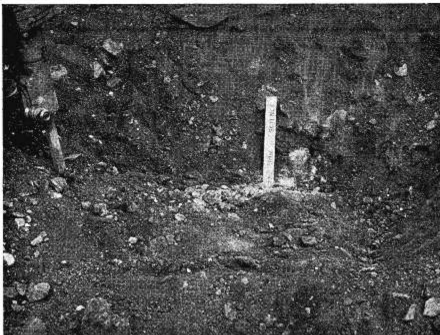
FIG. 3. Soil sample site 609-612, showing Jack-hammer excavation of exposed soil profile and frozen ground table.
