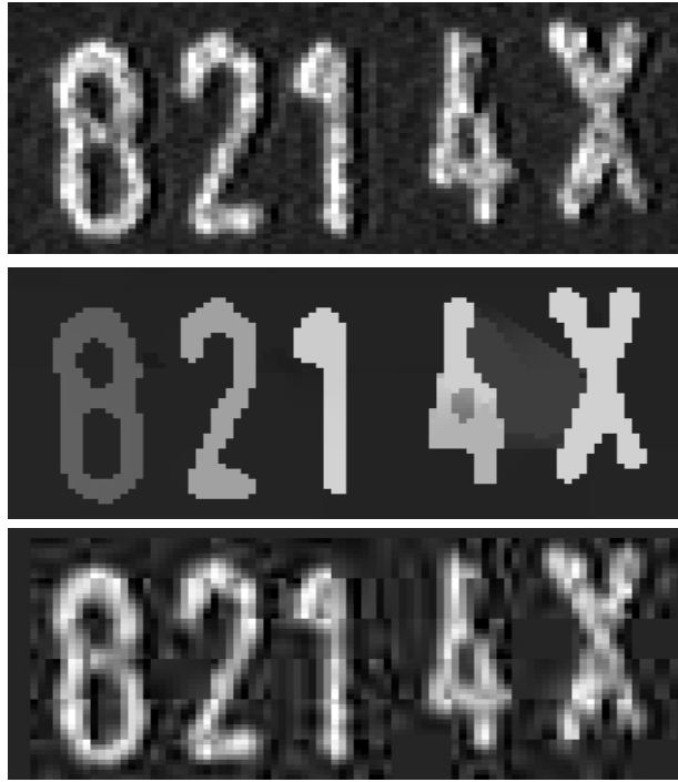
Figure 4: Numerals on a chip compressed by PSC with rate \leq 5\% . Top: original image; middle: PSC compression; bottom: compression by JPEG with comparable rate.
