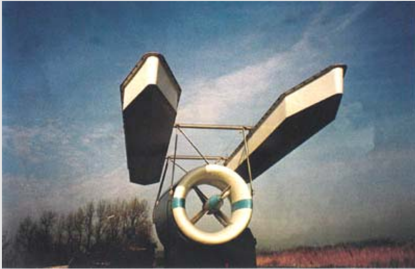
Tocardo Aqua75 free flow turbine Teamwork Technology, NL
