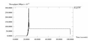
Figure 12. DCCP CCID2 with initial slow-start threshold value of 150
