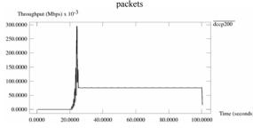
Figure 13. DCCP CCID2 with initial slow-start threshold value of 200 packets
