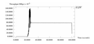
Figure 10. DCCP CCID2 with initial slow-start threshold value of 50 packets
