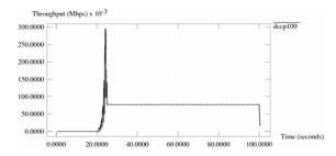
Figure 11. DCCP CCID2 with initial slow-start threshold value of 100 packets
