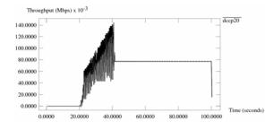
Figure 9. DCCP CCID2 with initial slow-start threshold value of 20 packets
