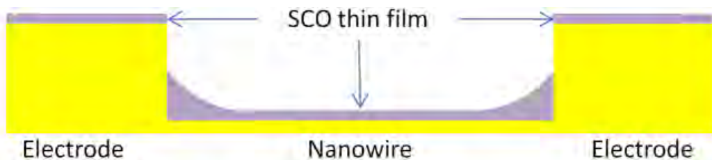
Figure 4.9: Scheme of the cross section of a nanowire circuit with the SCO thin film deposited on its surface.
