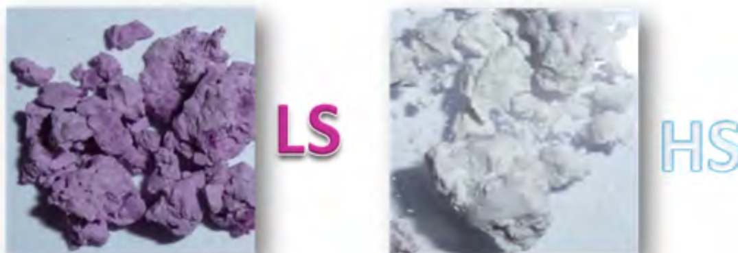
Figure 2.25: Images of the undoped [\text{Fe}(\text{hp}trz)_3](\text{OTs})_2 nanoparticle powder in the LS and HS states.
