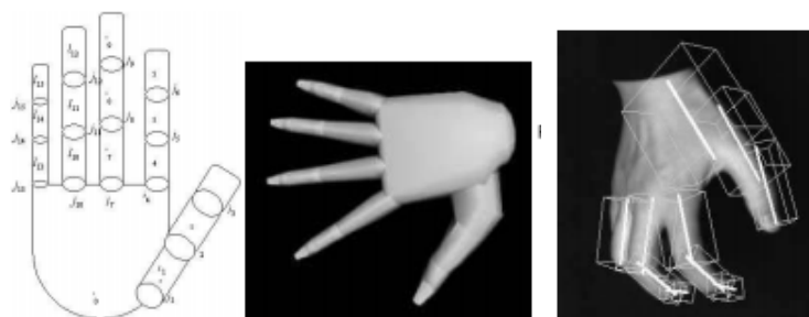
Figure 3.27: Hand tracking example using a 3D articulated model. Image extracted from [Wang 2009].
