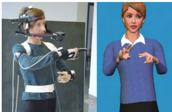
Figure 3.37: Generation from motion capture [Elliott 2000]
