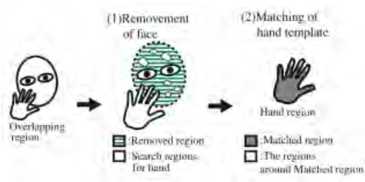
Figure 3.30: Illustrates the hand extraction using a template for hand and head before occlusion. Image extracted from [Tanibata 2002].
