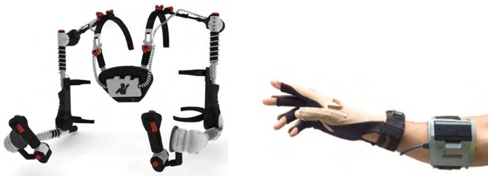
Figure 3.3: Mechanic sensors: exoskeleton Gypsy 7 (left) and CiberGlove II (right) 2
