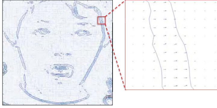
Figure 4.34: Head signature using gradient orientation
