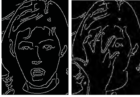
Figure 4.36: Contours from the face template and the image during occlusion.
