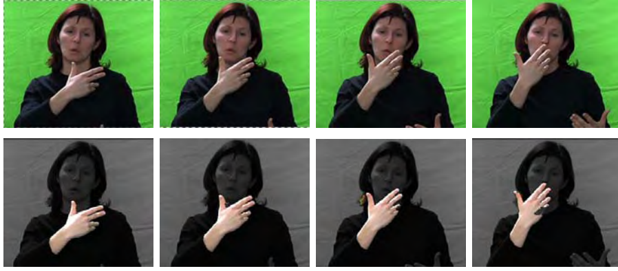
Figure 4.41: First row shows five consecutive frames in a sequence with hand over face occlusion. The second row shows the segmentation result. Pixels in dark grey or in black have been classified as belonging to the non hand class, otherwise they are shown in their natural colour.
