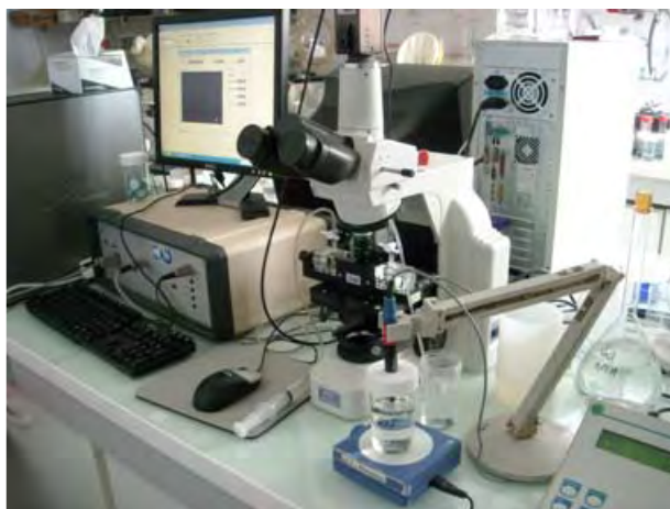
Fig. II. 7. Microelectrophoremeter CAD Instrumentation “Zetaphoremeter IV” Z 4000
