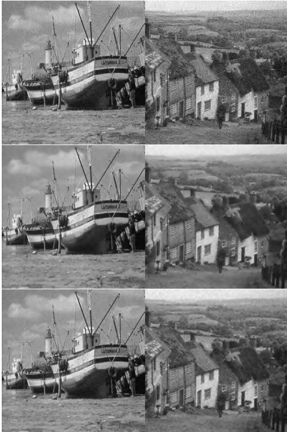
Figure B.3.: From top to bottom, Boat ( \sigma = 15 ) and Hill ( \sigma = 25 ) noisy images, restorations with \alpha = 1.5 and restorations with \alpha = 2.5 .
