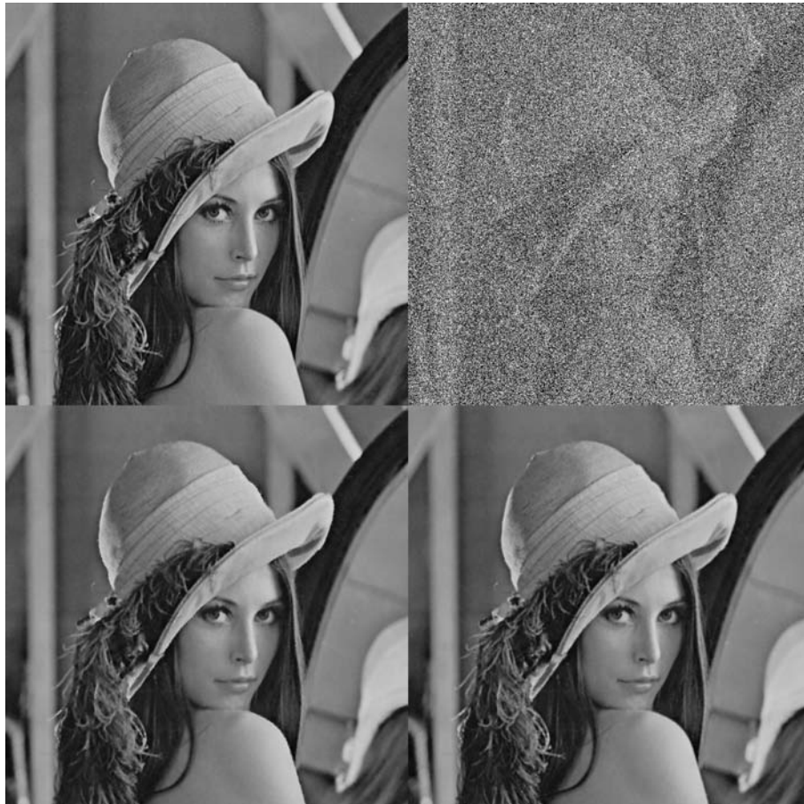
Figure 1.15.: From left to right, first line, original Lena image and noisy image (PSNR 6.30 dB), second line, isotropic restoration (PSNR 32.78 dB) and anisotropic restoration (PSNR 35.66 dB).
