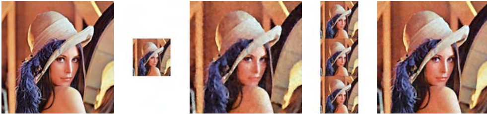
Figure 1.18.: Images from left to right: original, noisy filtered and sub-sampled, restored (PSNR 19.28 dB), three noisy filtered and sub-sampled, restored (PSNR 20.24 dB).
