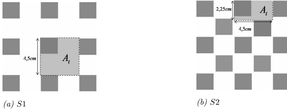
FIG. 2.19 – Configurations homogènes de rugosité : (a) S1 ( \lambda \approx 0.20 , A_t = 20.25 \text{ cm}^2 ) (a) S2 ( \lambda \approx 0.40 , A_t = 10.125 \text{ cm}^2 )
