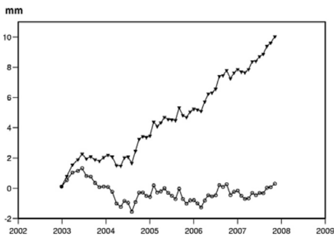
Fig. 1. Ocean mass change from GRACE over 2003–2008. The open circled curve is the raw time series. The black triangles curve corresponds to the GIA corrected time series.
