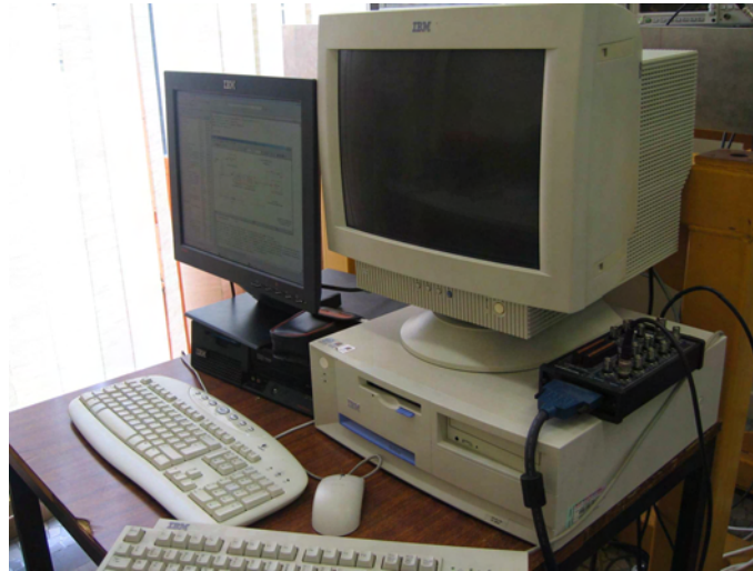
Figure 1.7: Detail view of acquisition system and xPC Target
