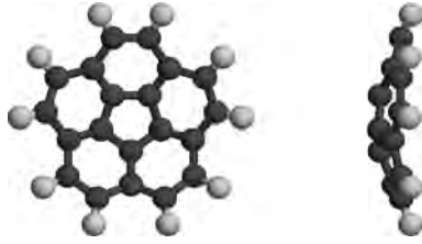
Figure 1. Structure of the corannulene molecule ( C_{20}H_{10} ). The central pentagonal carbon ring determines the bowl-shaped structure of the molecule, with a permanent dipole moment of 2.07 D along the symmetry axis.
