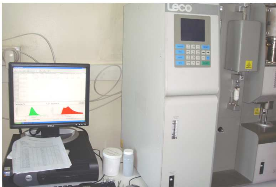
Figure 3-9: Photo of LECO CS200 analyzer (EPOC Analytical Laboratory, Bordeaux)
