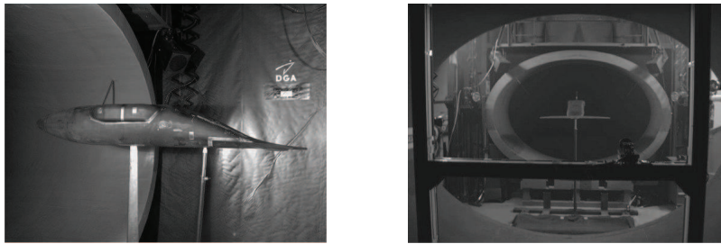
Fig. 2 View of the wind tunnel model and of its strut arrangement (left) and detail of the downstream 2C-PIV camera (right)
