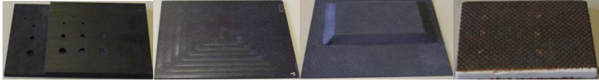
Figure 7: The four multi-layered and sandwich composite specimens
