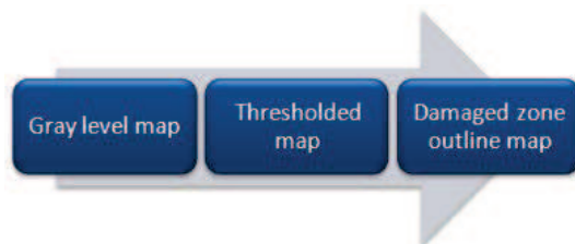
Fig. 7: Image processing procedure
