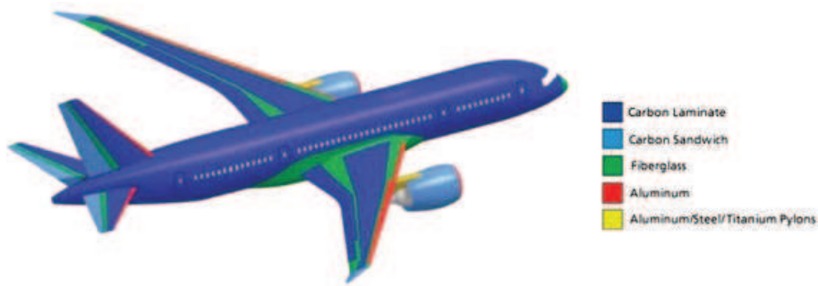
Figure 1. Boeing 787 material distribution [25].
