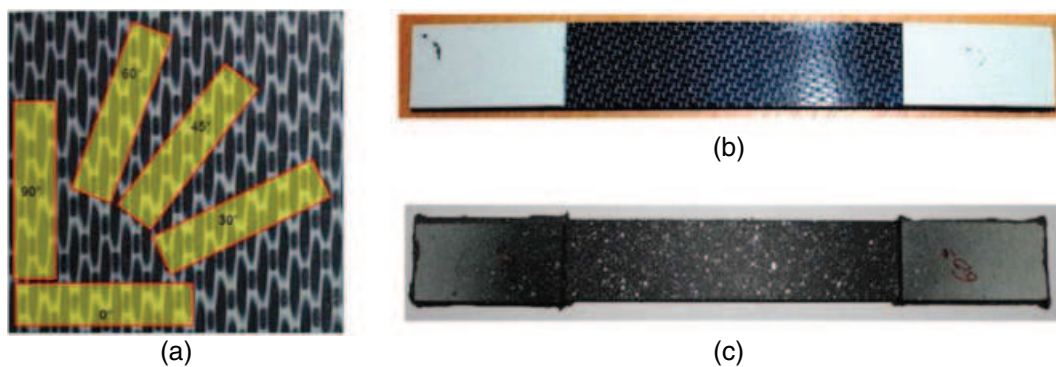
Figure 6. (a) Tensile samples orientation in the composite sheet, (b) tensile samples before testing and (c) grey level.
