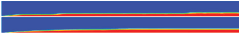
Fig. 8. Alignment of the interface on the mesh when VOF scheme is too compressive, for example with the Geo-Reconstruct scheme (top) compared with the HRIC scheme (bottom).
