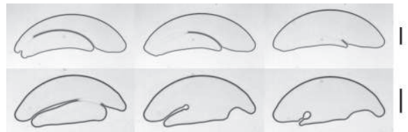
FIG. 6. Two sequences of film drainage. (Top three images) The liquid ligament is retracting at a constant velocity. (Bottom images) The film changes geometry halfway, and the fluid is collected in a rim. The scales on the right equal 1 cm.
