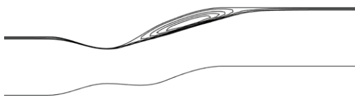
Fig. 5. Flow produced by the superposition of a bend and of a symmetric constriction. Streamlines calculated in the separated region with FLUENT.
