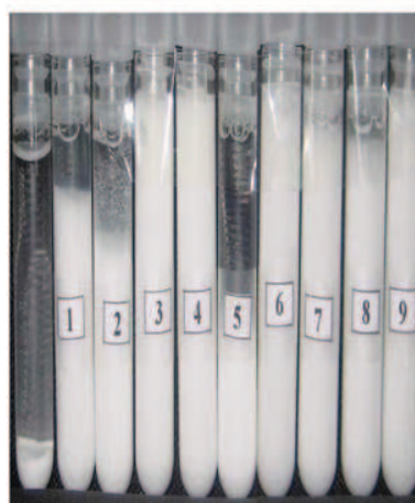
FIG. 12. Evolution of the clarification of the formulations as a function of time. The image shows the physical aspect of the “pure” suspension (5% ZnO) and of the various formulations after 8 weeks of storage. (Color figure available online.)
